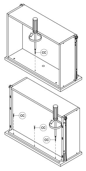
Pull out drawer slowly. Lock the drawer front panel into position using Wood Screws (cc).
