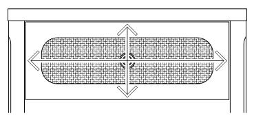
Insert the drawer into the main body, then adjust the drawer front panel left or right and up or down, until the drawer gaps look proportional.
