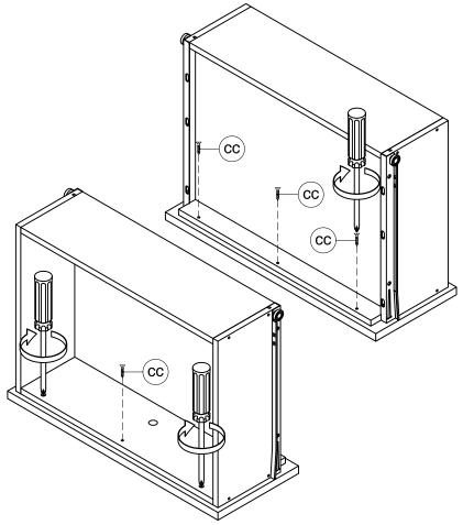
Pull the drawer open slowly and tighten the upper screws. Make sure the front panel does not move and lock the drawer front panel into position using Wood Screws (cc).
