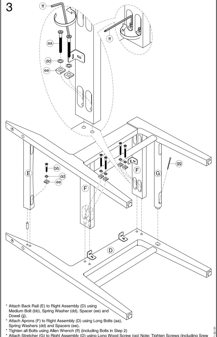
\* Attach Stretcher (G) to Right Assembly (D) using Long Wood Screw (gg) Note: Tighten Screws (including Srew in Step 2)
