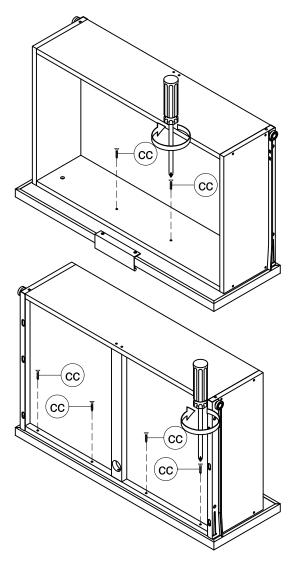
Pull out drawer slowly. Lock the drawer front panel into position using Wood Screws (cc).
