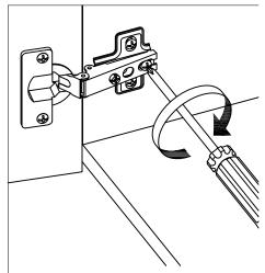
5.3. Tighten the back center screw.
