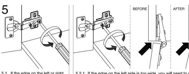
5.1. If the edge on the left or right are not balanced, loosen the back center screw.
