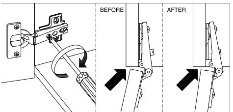
5.2.2. If the edge on the left side is too narrow, you will need to slide the doors slightly to the right by turning the front center screw counterclockwise.
