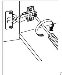
6.3. Tighten the back center screw.
